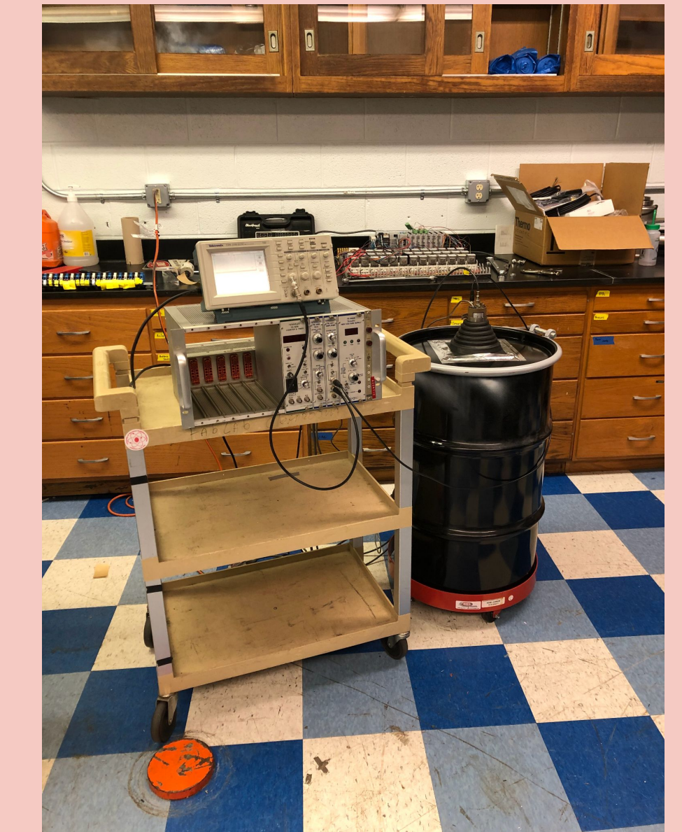
Figure 4: Fully assembled Cherenkov detector with Amperex xp2202b PMT
