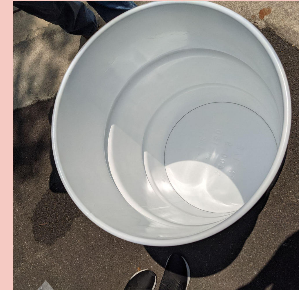
Figure 3: Inside of the detector barrel painted white to maximize reflectivity
